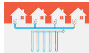
Ground source heat pump system with individual heat pumps in each dwelling.
