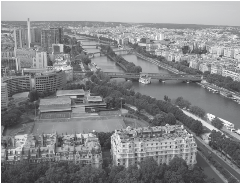
Figure 7.8. Narrowed channelized portion of a river through a city center where history has recorded huge floods. Continuous tree lines along both sides of the River Seine and on the island. Floodwaters draining a huge agricultural land, formerly forested, have inundated urban roads alongside the river. Low-rise buildings with large central courtyard (lower right) and a series of tiny courtyards (lower left); recreational fields and courts adjoining. Paris. R. Forman photo.
