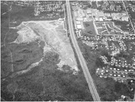
Figure 12.8. Dump filled with municipal solid waste and capped with clay layer. Eroded soil and chemicals have washed down to the left in several places. Small curved powerline through woods (left), multi-lane highway, detached single-unit housing (lower right), and small warehouse and truck terminal area (upper right). Suburban Boston. R. Forman photo.
