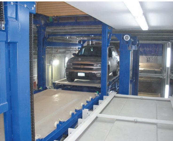
After traveling through the garage, vehicle and pallet are pushed into a storage space, where they are stored until the driver retrieves the vehicle.
