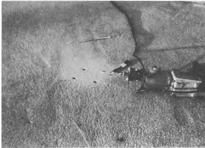
Figure 19-48: Obtaining concrete powder sample in field
