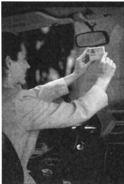
Figure 4- 4. AVI is becoming increasingly common for frequent parker entry/exit control. Photo courtesy Amtech.
