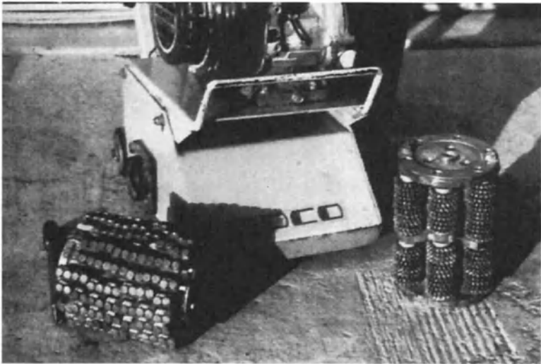
Figure 20-3: (a): Scarifier with cutter bits
