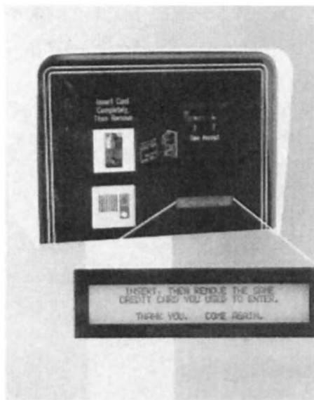
Figure 4-8. LED and LCD technology allows customized messages to be provided at PARC devices. Photo courtesy of Standard Parking Systems
