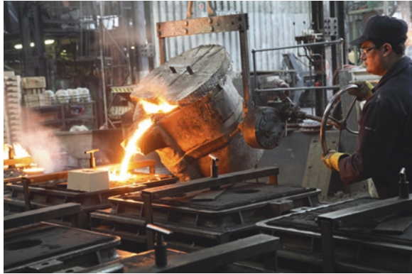
Fig. 5.2 Castings being made from pouring molten metal. Vanguard Foundry Ltd, West Midlands, UK
