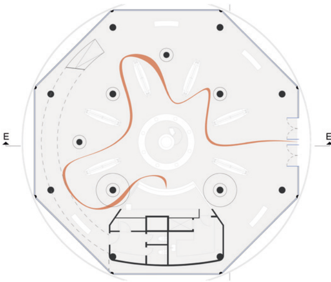
Fig. 1.45 Plan of Placebo Pharmacy in Athens. Designed by Klab Architecture/Konstantinos Labrinopoulos, 2010. Brown line indicates public circulation from the entrance
