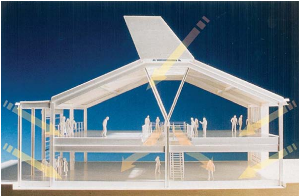
Section of model to illustrate the daylighting
